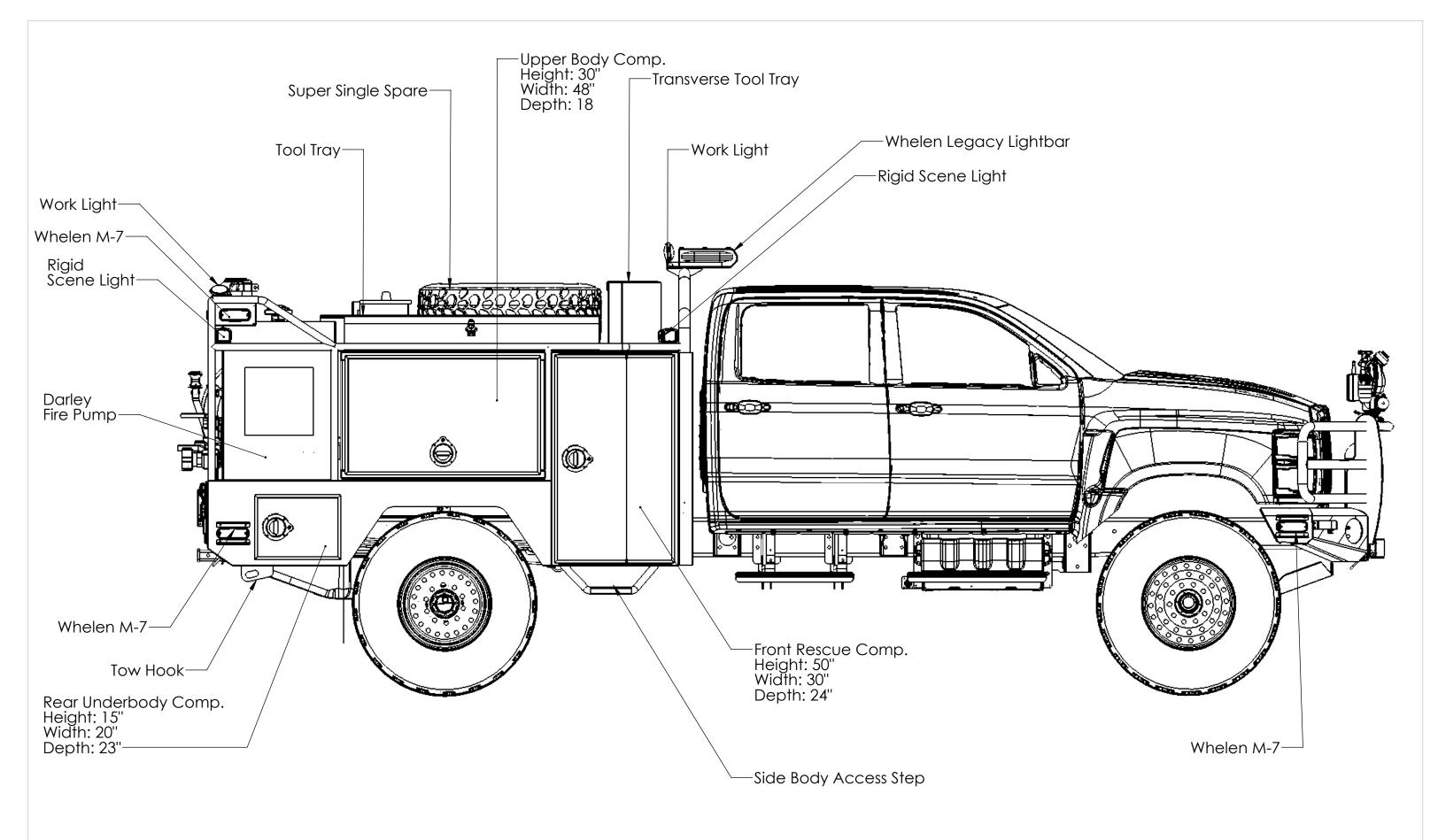
AND ARE SUBJECT TO MINOR DEVIATIONS AS MAY OCCUR OR BE NECESSARY IN CONSTRUCTION MINOR DETAILS NOT SHOWN
