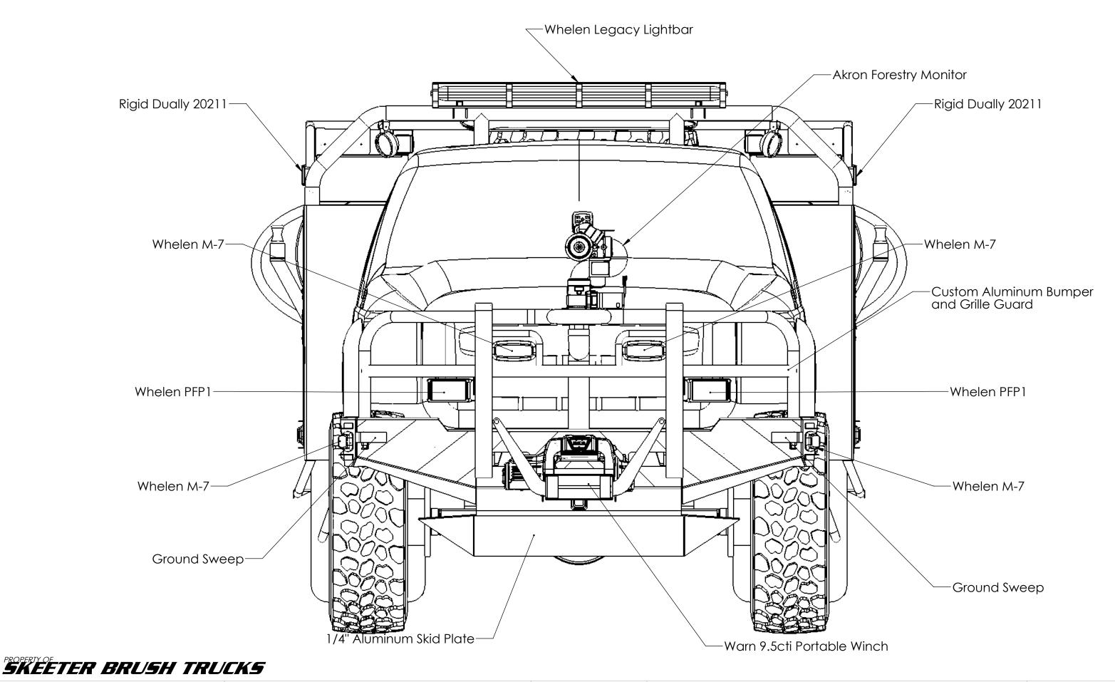
NOTE: DETAILS AND DIMENSIONS SHOWN ARE APPROXIMATE PREPARED FOR: AND ARE SUBJECT TO MINOR DEVIATIONS AS MAY OCCUR OR BE NECESSARY IN CONSTRUCTION
