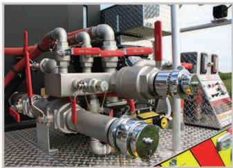
Stainless Steel Plumbing
