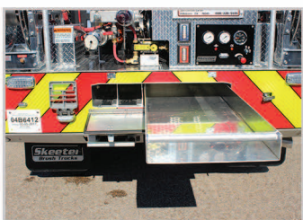
Hard Suction Storage
